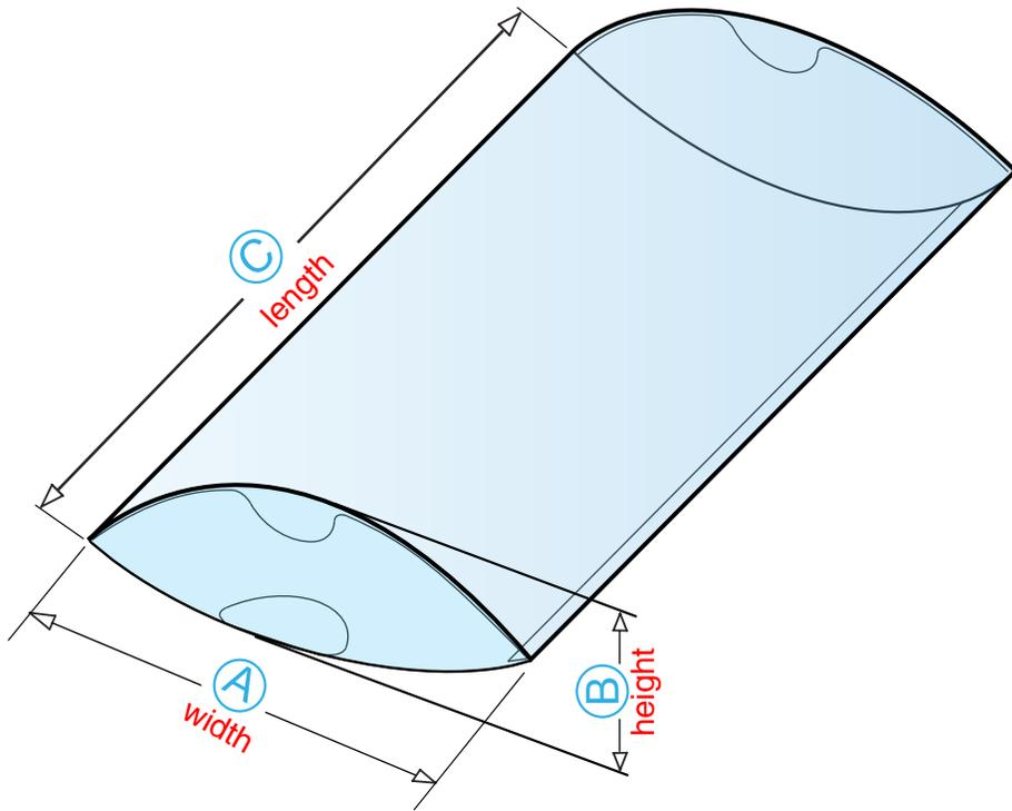
Pillow Packs are a cost-effective style of packaging, typically used for products of shallow depth or for bulk packs of small items. A wide variety of features can be included to provide added utility, i.e.: thumb locks, standing bottoms, or hang tabs.
