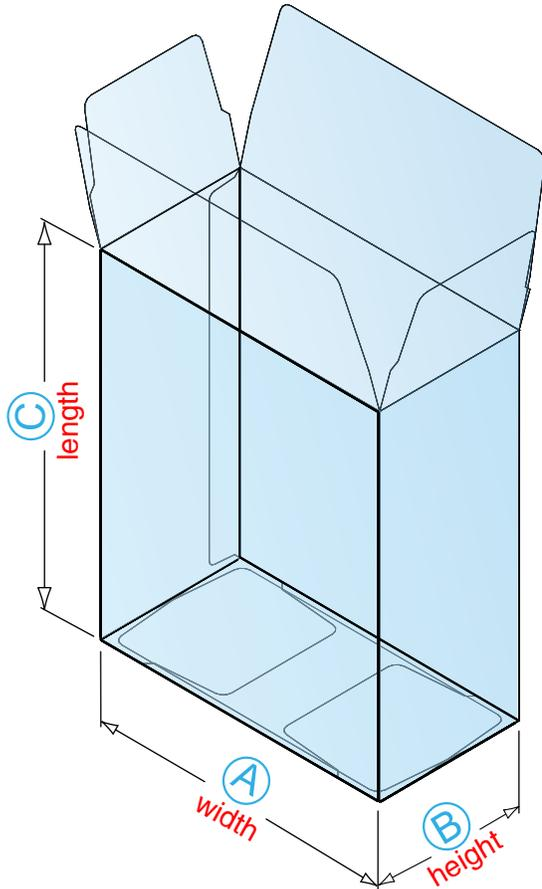
The Seal End carton is typically erected, filled and sealed on automated packaging equipment. Since the top and bottoms are glued closed, it offers tamper evidence as compared to tuck style cartons.
