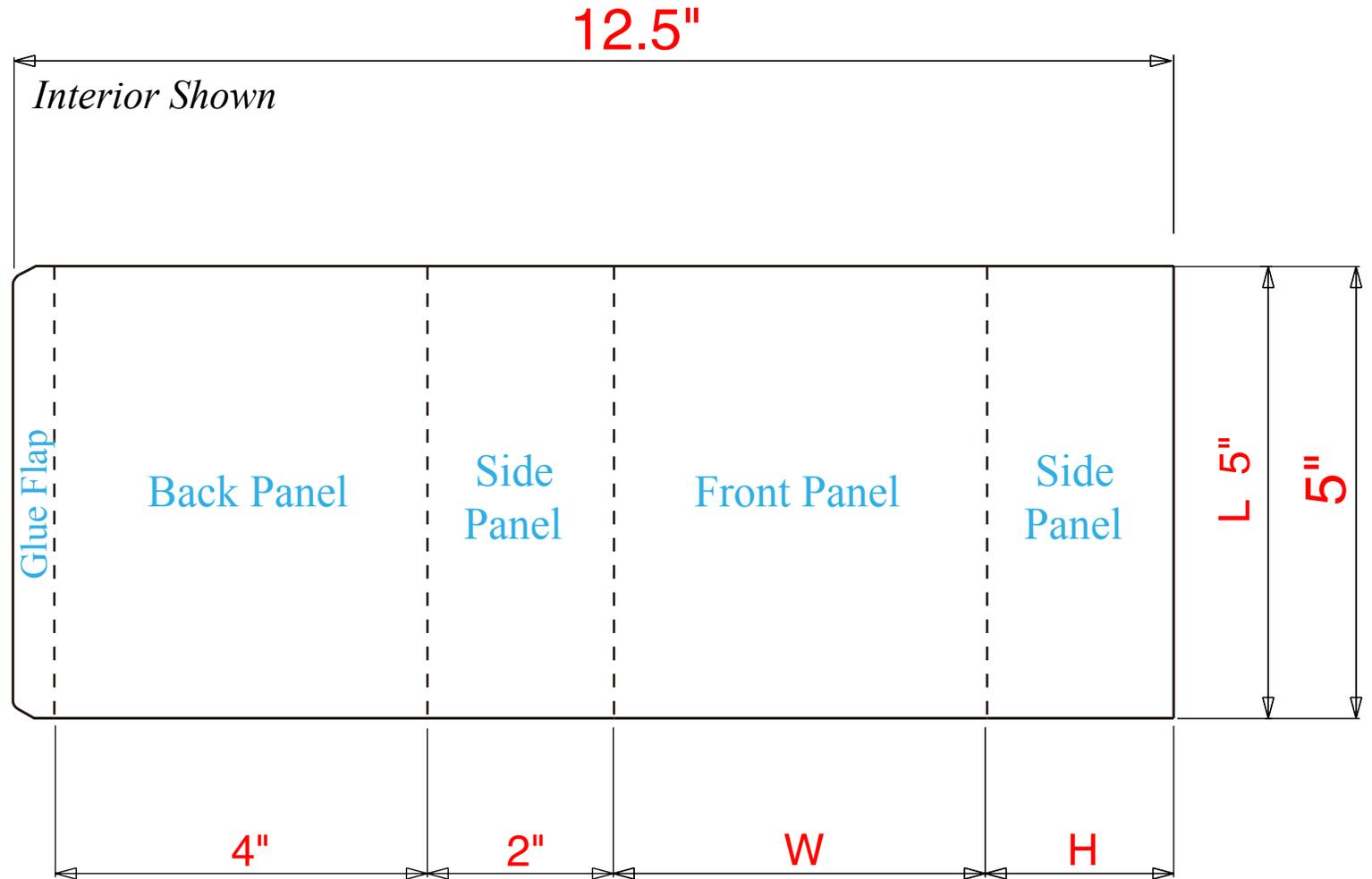
A Sleeve is used in combination with another packaging component. It's frequently used as a slip-on cover for a paperboard carton or tray, or an open set box structure. Sleeves can also be used in combination with injection molded or vacuum-formed plastic end caps or inserts.
