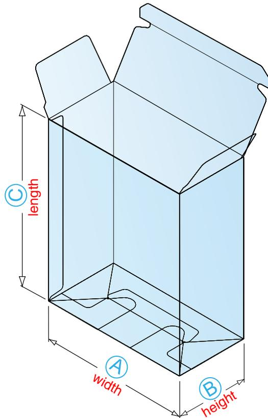
123-Bottom cartons are designed for efficient hand set-up and loading. Although not as efficient as Auto-Bottom cartons, this carton style is also used when faster set-up is desired but production volume or the package's contents are not suitable for automatic packaging equipment.
